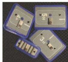
Figure 1. For hyperthermia, heat was induced electromagnetically by using these microelectrode applicators.
